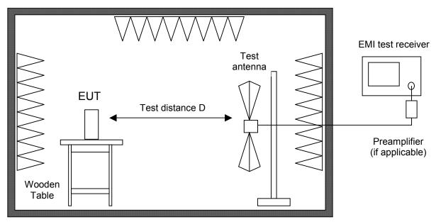
Alternate test site (semi anechoic room)
