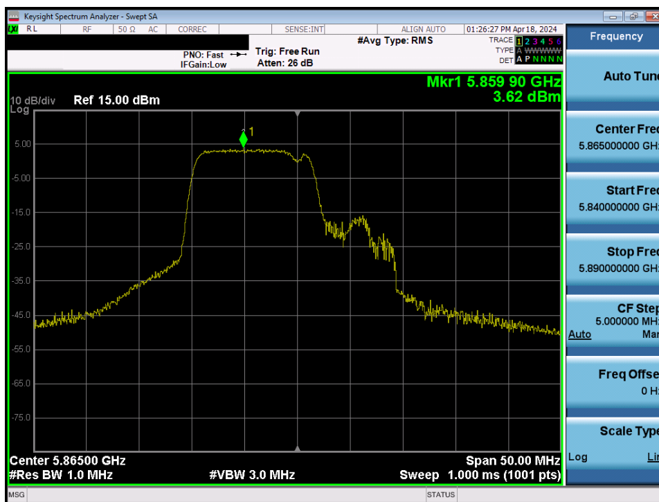
Plot 7-178. Power Spectral Density Plot MIMO ANT2 (20MHz BW 802.11be – 106+26 Tones (UNII Band 4) – Ch. 173)
