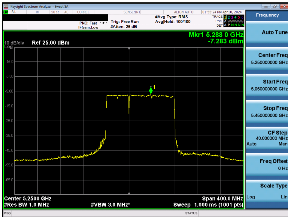
Plot 7-166. Power Spectral Density Plot MIMO ANT2 (160MHz BW 802.11be – 996+484 Tones (UNII Band 1/2A) – Ch. 50)
