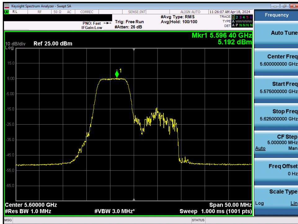
Plot 7-170. Power Spectral Density Plot MIMO ANT2 (20MHz BW 802.11be – 52+26 Tones (UNII Band 2C) – Ch. 120)
