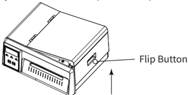
2. After the cover is opened, press the arrow on the cover opening button, move the cover opening button upward, and lift the movement group to replace the paper.
