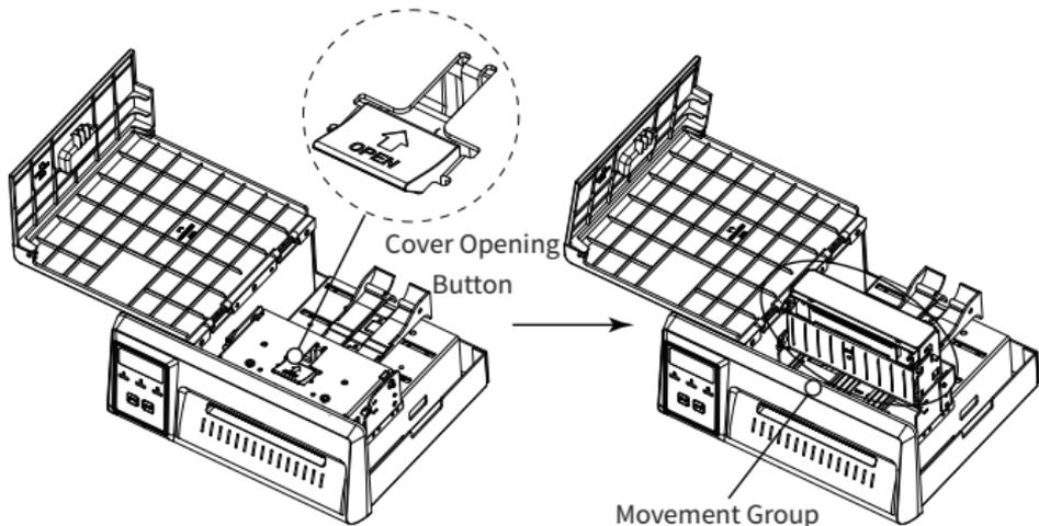
3. Press the movement group down and the movement group can be reset. Pass the paper through the paper limiter from the rear of the printer. When the paper passes through the middle of the movement group, the sensor detects the paper, and the printer can automatically feed the paper.
