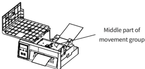
4. According to the width of the paper, adjust the position of the paper limiter by moving it .
