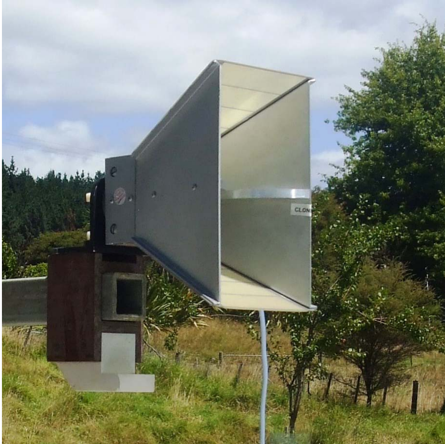
EMCO 3115 Horn Antenna (1 – 18 GHz)
