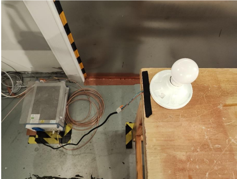
Photograph 2: Set-up for measurement of radiated emission
