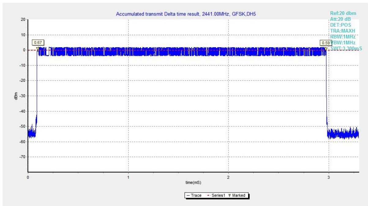
Fig. 60 Time of Occupancy(Dwell Time) (GFSK, Ch39)
