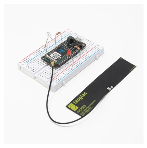
The Particle Boron is a mesh and Bluetooth development kit designed for building connected projects and products. To set up the device you'll need an Android or iOS mobile phone and a connection to the internet.
