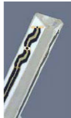
Figure 2.3 Probe Thick-Film Technique
