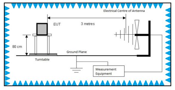
Test setup diagram for Radiated Spurious Emissions testing (below 1GHz):
