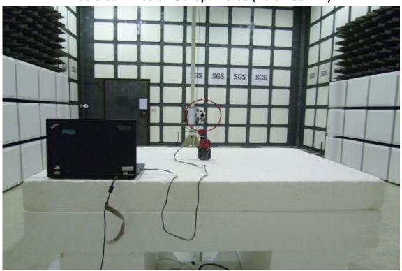
Radiated Emission Set up Photos (Below 1GHz)
