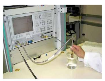
Tissue used during the SAR assessment is calibrated prior to the measurement process. APREL Laboratories use the co-axial probe method for all tissue calibration exercises. Tissue which is being used over a period of 24 hours is recalibrated to ensure that no change to the dielectric properties will affect the SAR measurement process. The table below provides details of the tissue results from the equivalent dielectric calibration.
