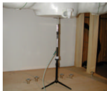
Figure 12.1 Dipole Validation Test Setup
