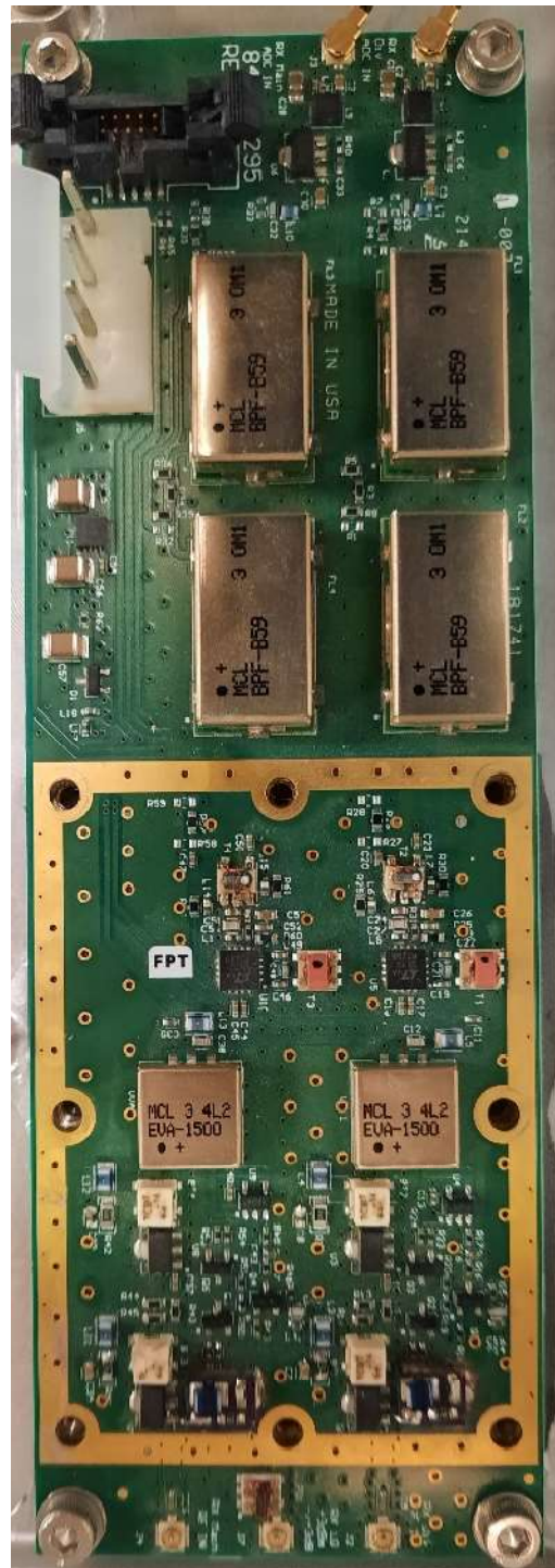
Receive Board – Top - Shield Removed
