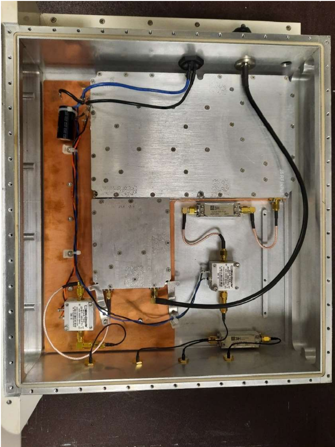
PA Module Bottom Cover Removed
