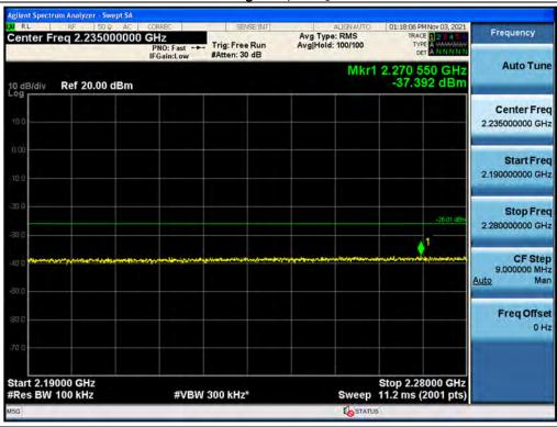
Antenna 1 / High Edge + 100 MHz ~ 10 GHz / B66 LTE 20 MHz 1 Carrier + B66 LTE 10 MHz 1 Carrier [2 Carrier] / Non-Contiguous / QPSK
