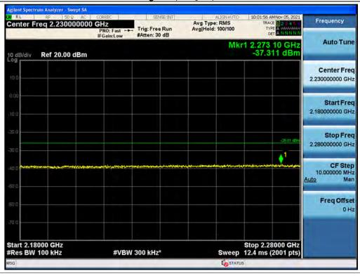
Antenna 1 / High Edge + 100 MHz ~ 10 GHz / B66 LTE 20 MHz 1 Carrier + 5G NR n66 5 MHz 1 Carrier [2 Carrier] / Contiguous / QPSK / Low
