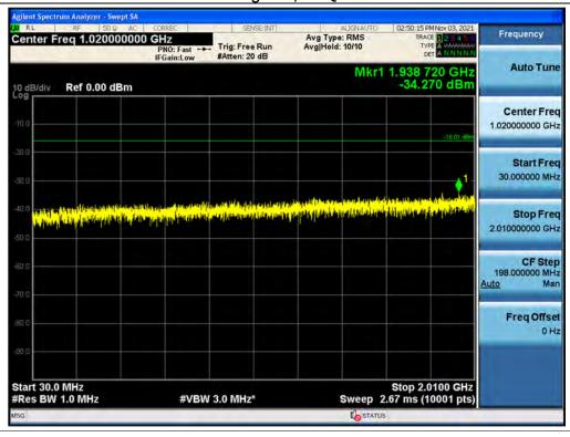
Antenna 1 / Low Edge - 100 MHz ~ Low Edge / 5G NR n66 20 MHz 1 Carrier + 5G NR n66 10 MHz 1 Carrier [2 Carrier] / Non-Contiguous / 64QAM
