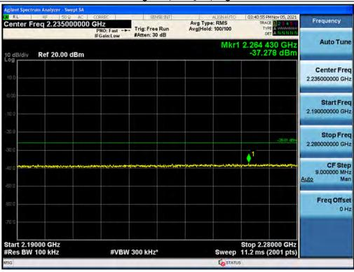
Antenna 1 / High Edge + 100 MHz ~ 10 GHz / B66 LTE 20 MHz 1 Carrier + 5G NR n66 10 MHz 1 Carrier [2 Carrier] / Contiguous / QPSK / Middle
