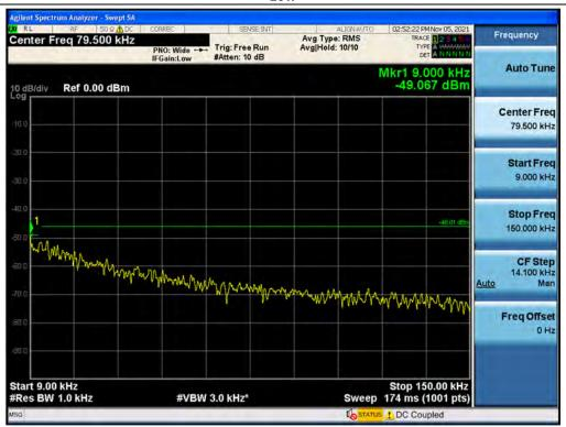
Antenna 1 / 150 kHz ~ 30 MHz / B66 LTE 20 MHz 1 Carrier + 5G NR n66 10 MHz 1 Carrier [2 Carrier] / Contiguous / 16QAM / Middle
