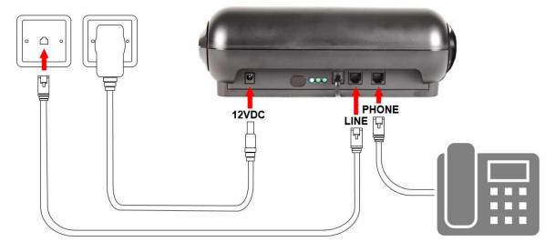
Figure 7: GPS Base Unit Connections
