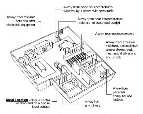
Figure 6: Positioning the GPS Base Unit
