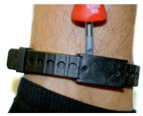
Figure 8: Prying Apart the Locking Clip of the RF Transmitter
