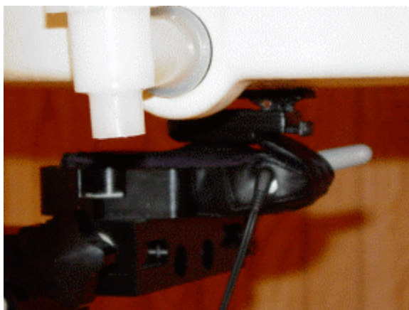
Figure 10.5 KE414 body SAR setup (with leather case)
