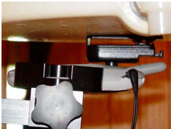
Figure 10.9 KE424C body SAR setup (with belt clip)
