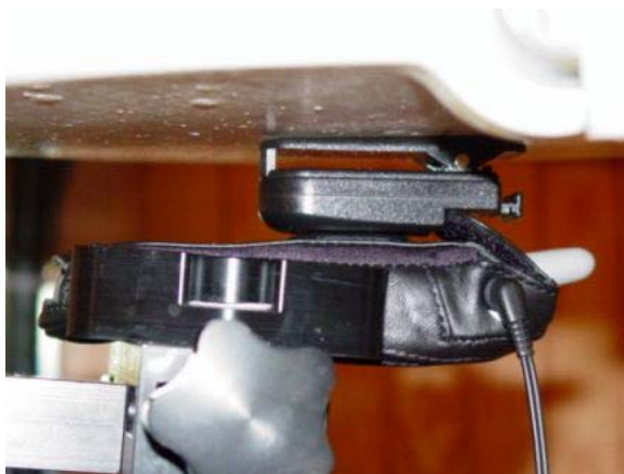
Figure 10.10 KE424C body SAR setup (with leather case)
