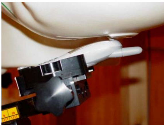
Figure 10.8 KE424C phone against the head (left tilt position)
