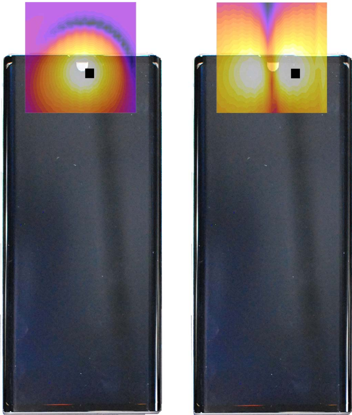
Figure 16-5 T-Coil Scan Overlay Magnetic Field Distributions
