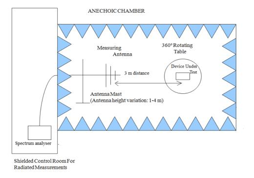
Radiated measurements setup f > 1 GHz
