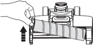
Remove the brush roller by grabbing the brush roller tab and pulling upward.
