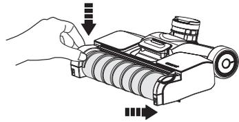
Replace the brush roller by inserting the brush roller end into the right side of the holder, then lock the pull tab into place by pressing downward.
