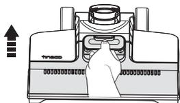
Grab the front handle while pressing the button and pull upward to remove.
