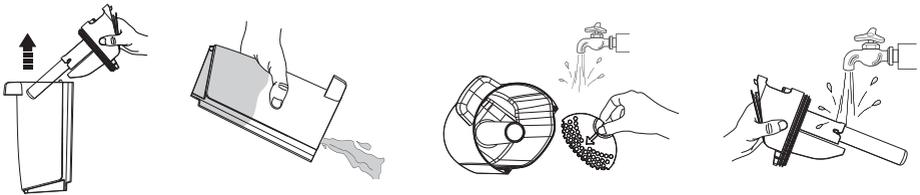
If the filter and the floater have been blocked, rinse with water.
