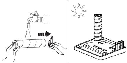
Remove the hair and debris wrapped around the roller and rinse with water (brush roller tab can be removed). Replace the brush roller back onto the storage tray, and allow it to dry completely before reinstalling.
