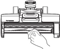
Remove hair and debris from the brush roller chamber and the opening with a tissue or a damp cloth.
