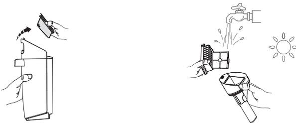
Grasp recessed area on each side of the filter and pull upward. Rinse under running water and must be completely dry before recombining with the lid of the DWT.
