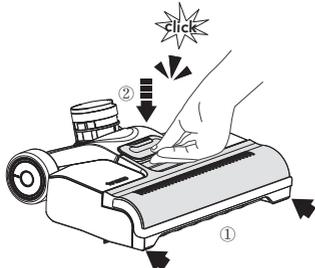
When replacing, always latch the brush cover into place to avoid leakage.
