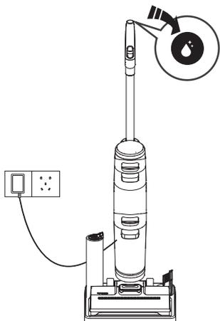
1. Place the appliance on the storage tray and plug in. Press the self-cleaning button and begin the process.
