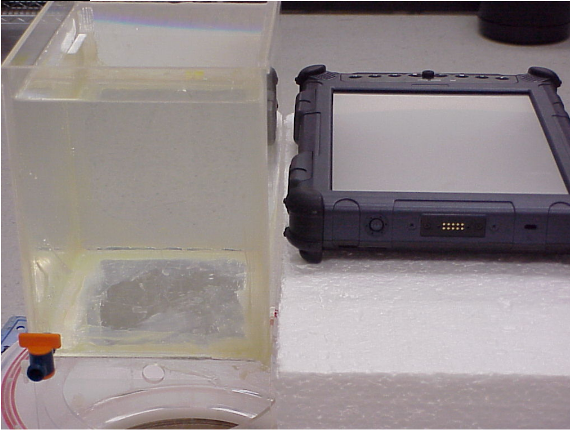
Photo 4. GPRS antenna bystander position
