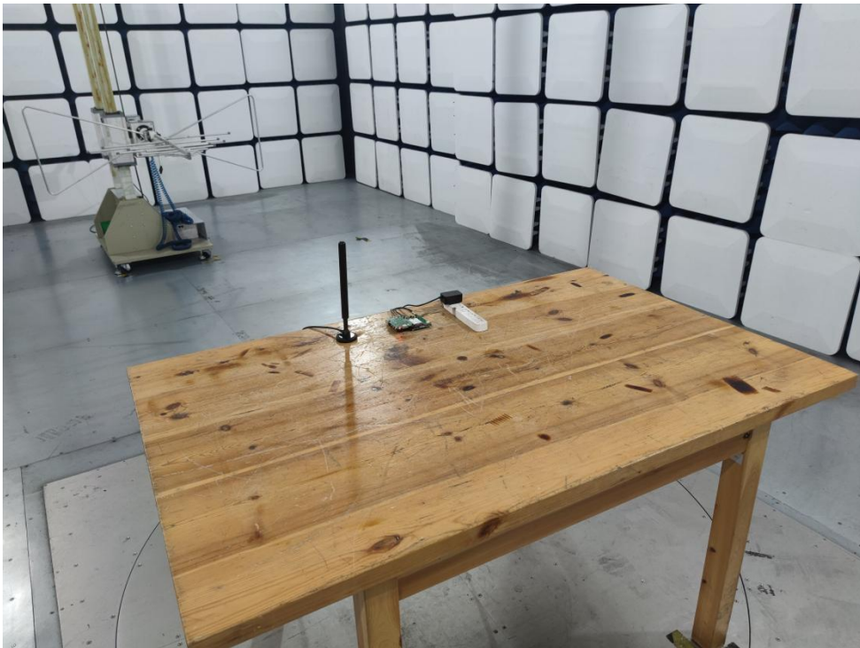
Photo of Radiation Emission Test
