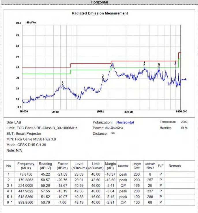
Note:1).Level (dBµV/m)= Reading (dBµV)+ Factor (dB/m)
