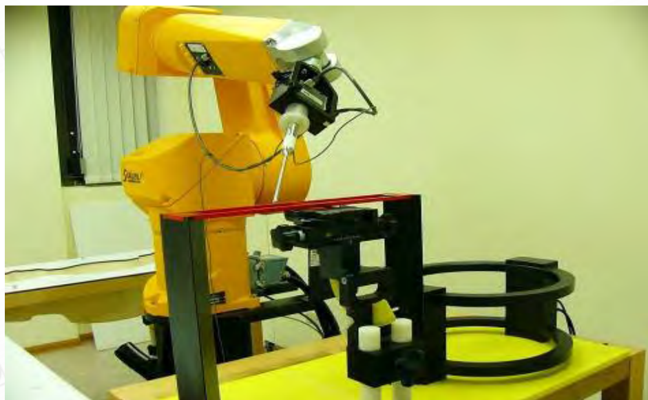
Fig. 1 Photograph of the DASY 5 measurement system
