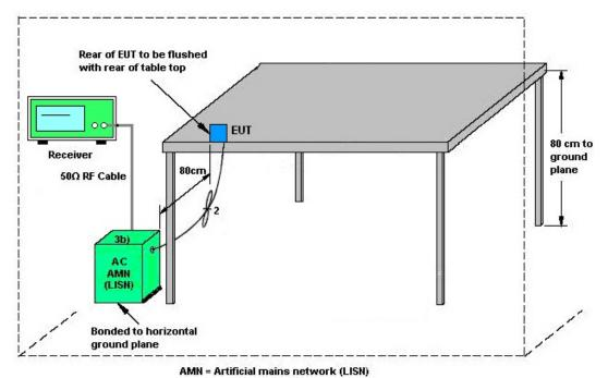
AE = Associated equipment EUT = Equipment under test
