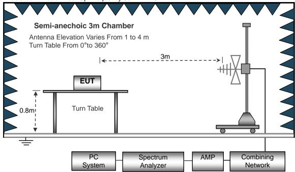
(C) Radiated Emission Test-Up Frequency Above 1GHz
