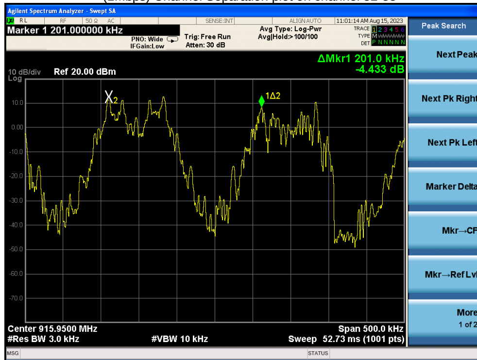
(1Mbps) Channel Separation plot on channel 102-103
