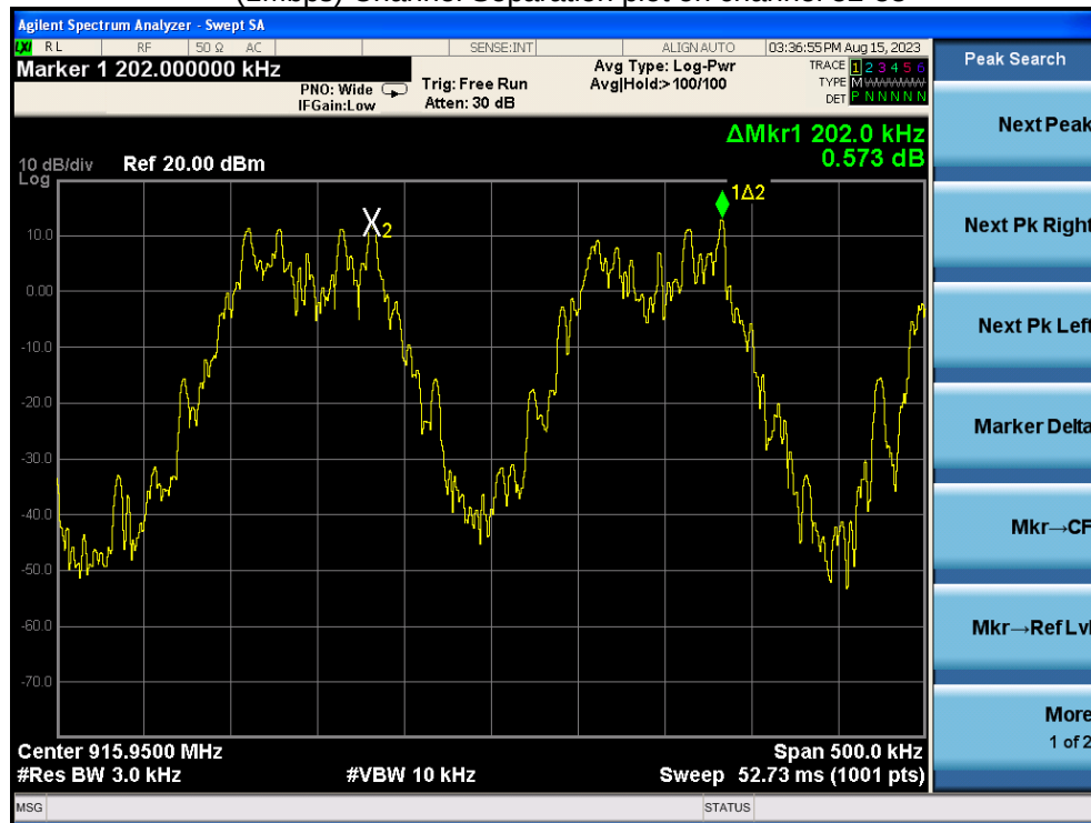
(1Mbps) Channel Separation plot on channel 102-103
