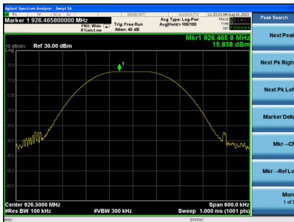
Peak output Power plot on channel 103 (1Mbps)
