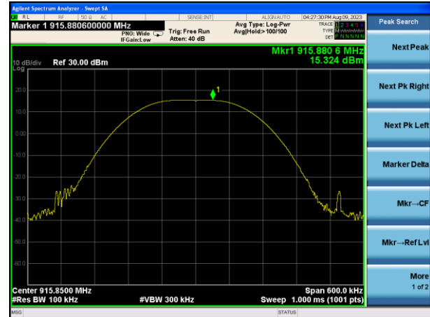
Peak output Power plot on channel 52 (1Mbps)
