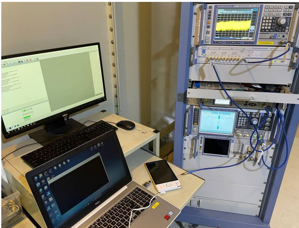
Conducted RF Output Power Test Setup
