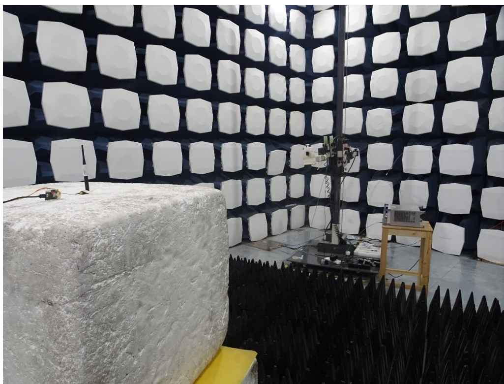
Picture 1 Radiated Emission Transmitter Unwanted Emissions Test Setup
