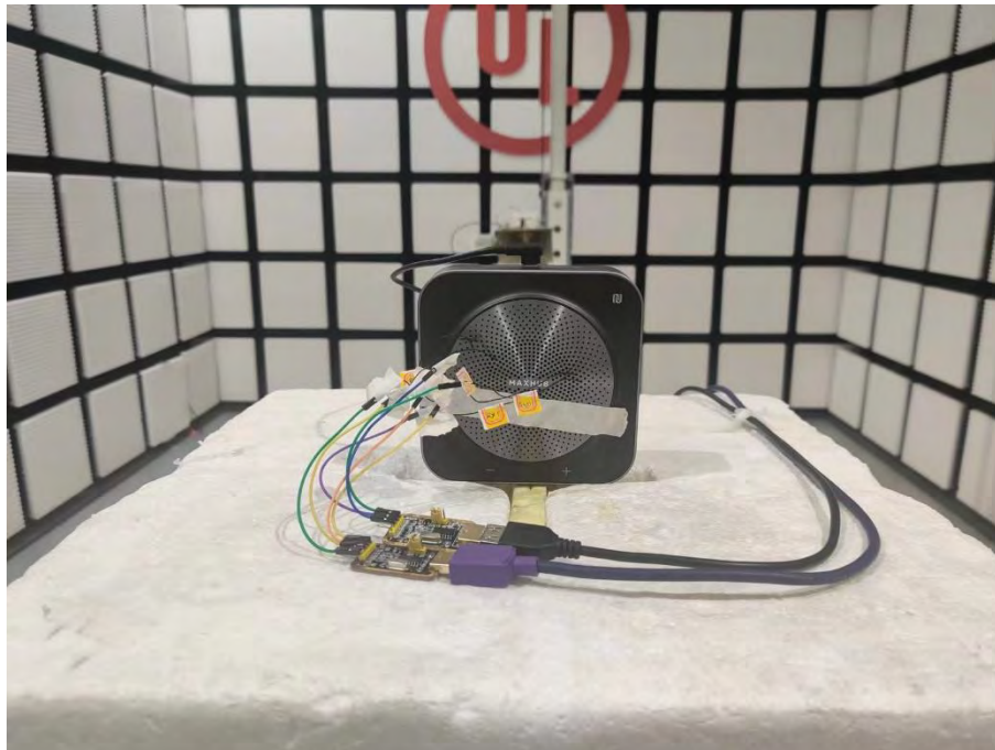
Radiated Disturbance Setup (Above 1 GHz – Z axis)
