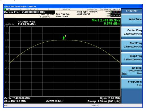
Test Plots (8DPSK) Peak Power (CH.0)
