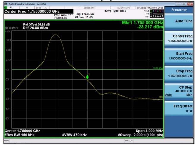
LTE B4\_15 M\_Band Edge\_High\_QPSK\_1RB
