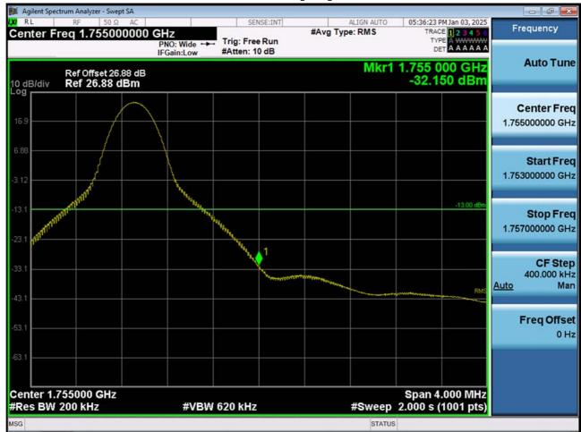
LTE B4\_20 M\_Band Edge\_High\_QPSK\_1RB
