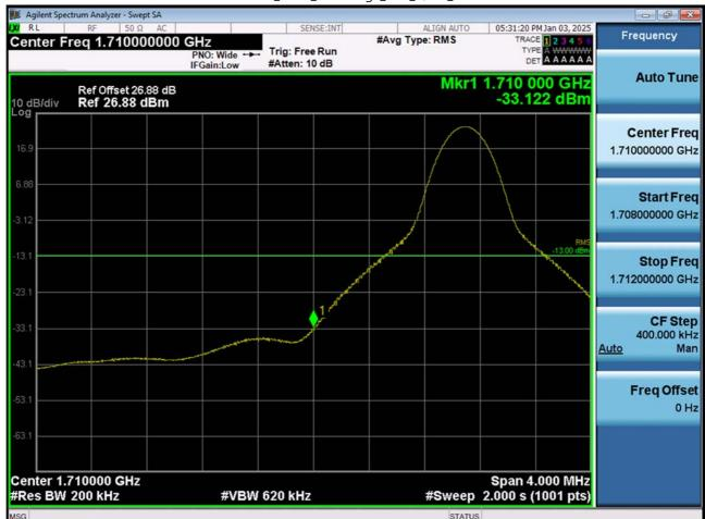
LTE B4\_20 M\_Band Edge\_Low\_QPSK\_1RB
