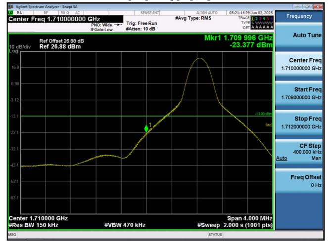
LTE B4\_15 M\_Band Edge\_Low\_QPSK\_1RB
