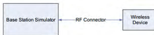
Figure 9.1 Power Measurement Setup
