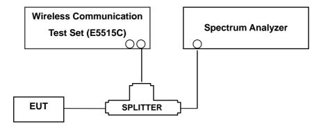
(Configuration of conducted Emission measurement)
