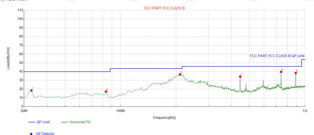
Suspected List Freq. Factor Reading Level Limit Margin Height Angle NO. Polarity [MHz] [dB] [dBµV/m] [dBµV/m] [dBµV/m] [dB] [cm] [°] 32.912913 -15.12 33.57 18.45 40.00 21.55 100 230 Horizontal 83.403403 -18.05 35.29 17.24 40.00 22.76 100 Horizontal 3 210.60060 -14.88 51.69 36.81 43.50 6.69 100 219 Horizontal 445.57557 -8.66 46.00 4 42.99 34.33 11.67 100 42 Horizontal 742.69269 5 -3.41 43.25 39.84 46.00 6.16 100 211 Horizontal -1.49 891.25125 40.00 38.51 46.00 7.49 100 300 Horizontal
