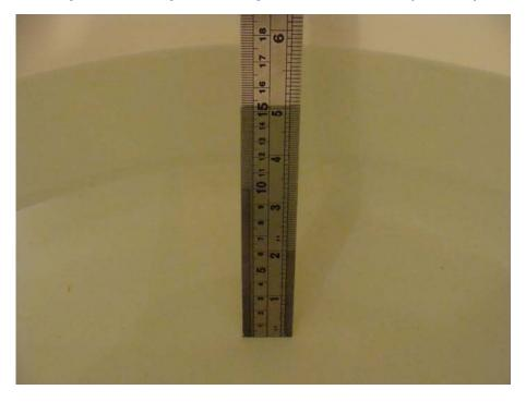
Depth of the liquid in the phantom-Zoom In (5GHz)
