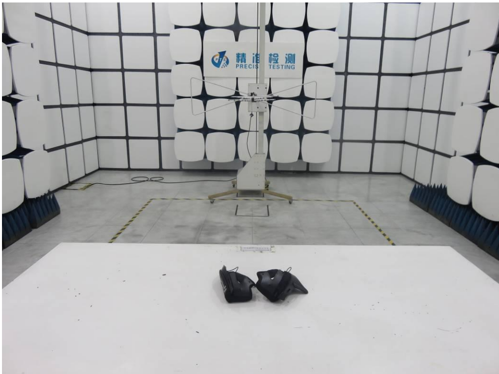
FCC RADIATED EMISSION TEST SETUP
