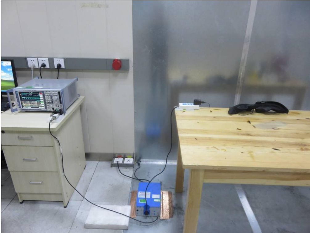
FCC RADIATED EMISSION TEST SETUP
