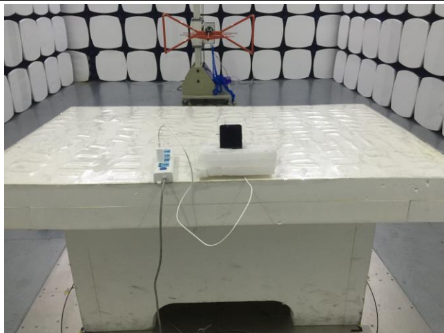
Conducted Emissions Test Setup Front View
