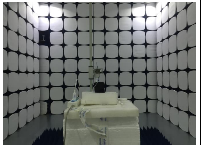
Radiated Spurious Emissions Test Setup Above 1GHz
