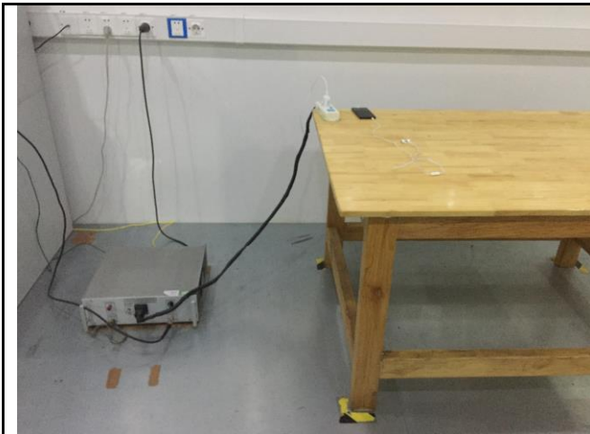
Conducted Emissions Test Setup Front View
