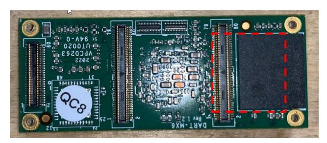
Note: The red outline shows the PQG-XREADER device boundaries. It does not include the Variscite DART-MX6 computer module.
