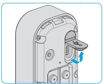
**Q2** Plug in the provided power cord into the USB-C port.
