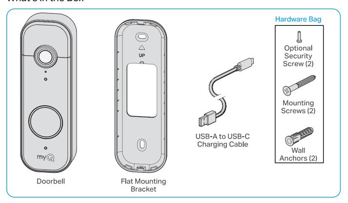
**TIP:** Wood screws are provided to attach the mounting bracket to your door frame. If you are mounting the doorbell on a wall made of stucco, brick or concrete, you will need the plastic anchors.
