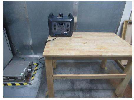
Radiated Emissions (9kHz-30MHz)
