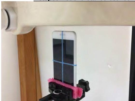
Fig.12 EUT Bottom side to flat phantom
