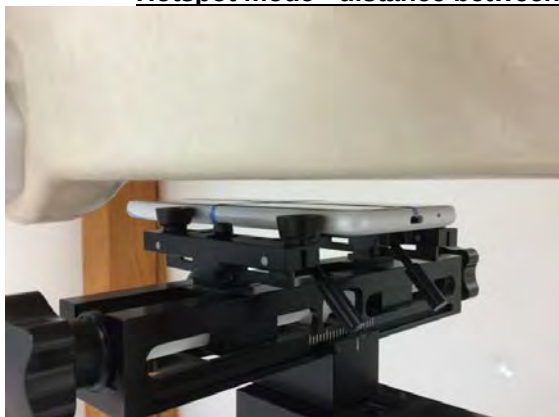
Fig.9 EUT Front side to flat phantom
