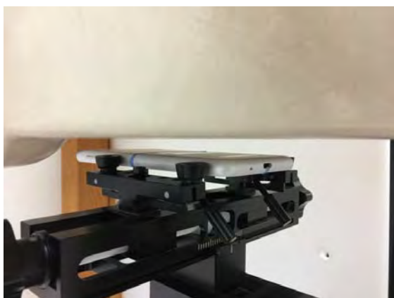
Fig.8 EUT Back side to flat phantom
