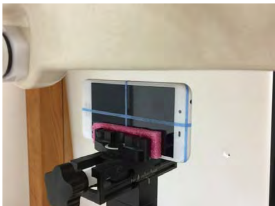
Fig.14 EUT Left side to flat phantom
