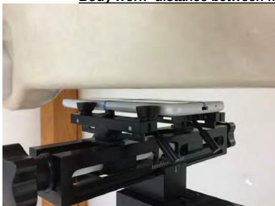
Fig.7 EUT Front side to flat phantom
