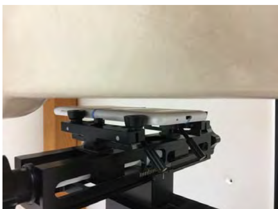
Fig.10 EUT Back side to flat phantom
