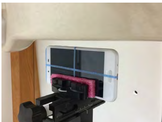
Fig.13 EUT Right side to flat phantom
