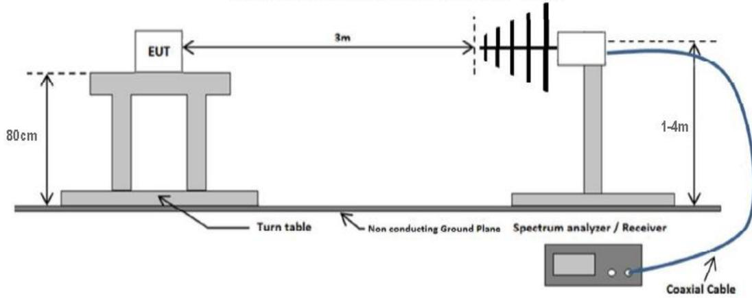
**Radiated emissions test setup above 1 GHz**
