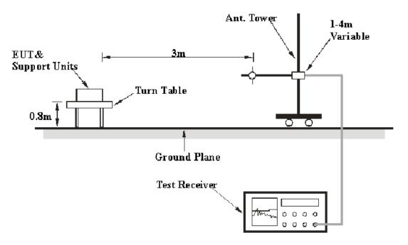
Note: for below 30MHz, the antenna height is 1m.
