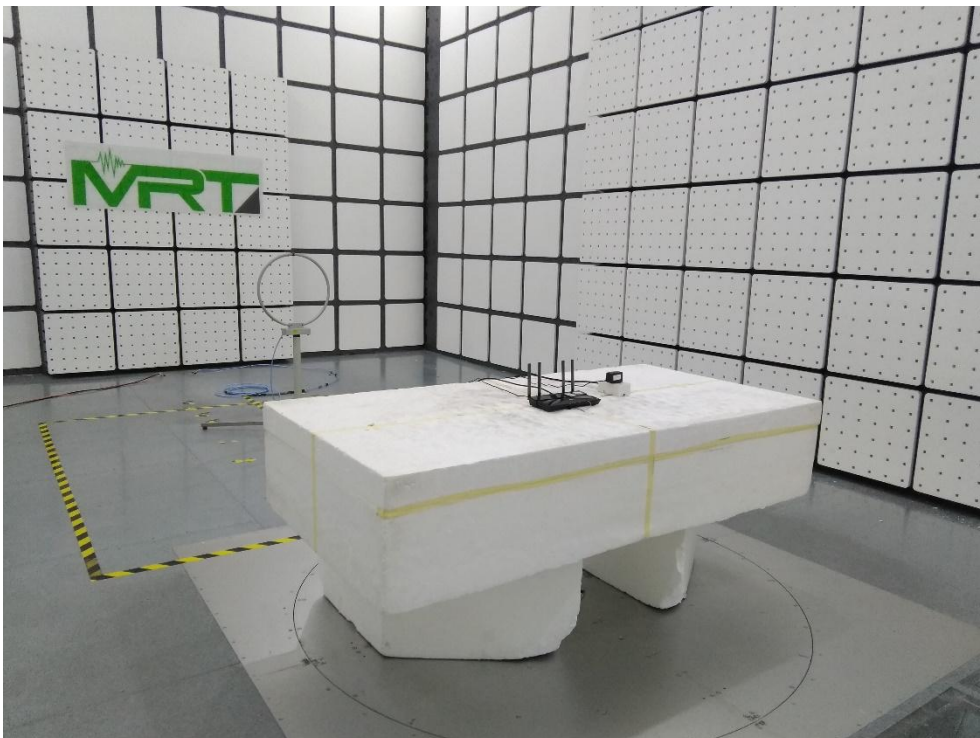
Description: Radiated Emission Test Setup for 9kHz~30MHz
