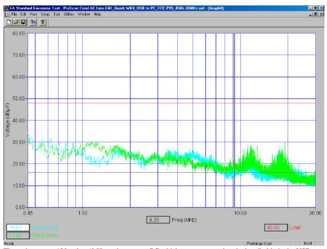
The ac input was 120 volts, 60 Hz to the support PC which was connected to the handheld via the USB data cable.
