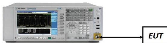
Figure 7-5. Test Instrument & Measurement Setup
