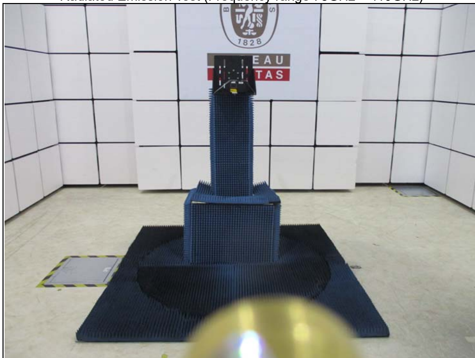
Radiated Emission Test (Frequency range 110GHz ~ 170GHz)
