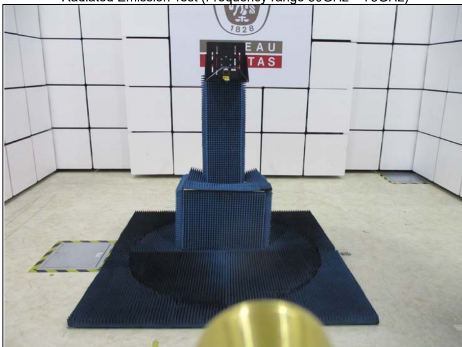
Radiated Emission Test (Frequency range 50GHz ~ 75GHz)
