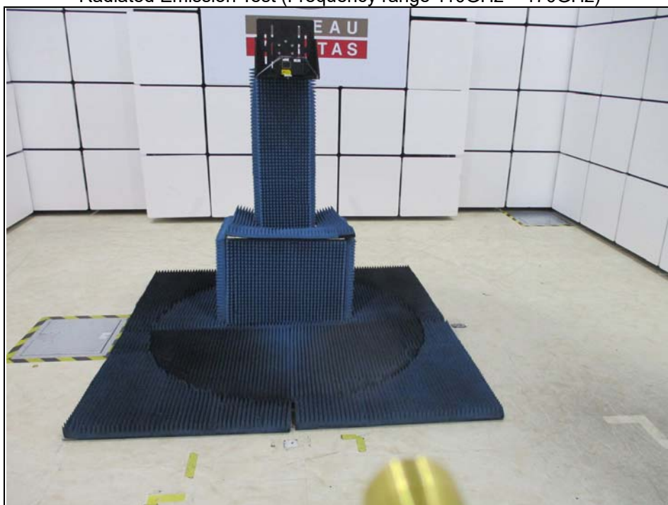
Radiated Emission Test (Frequency range 110GHz ~ 170GHz)
