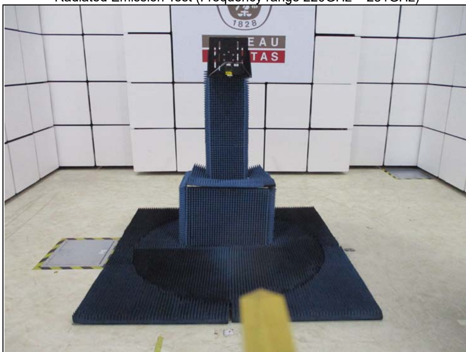
Radiated Emission Test (Frequency range 220GHz ~ 231GHz)
