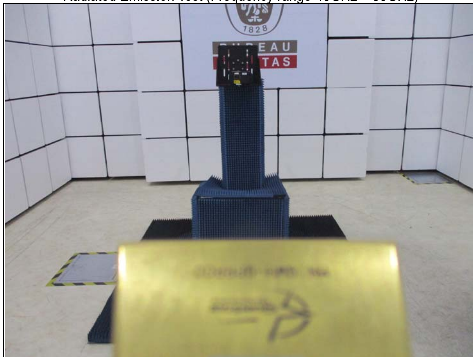
Radiated Emission Test (Frequency range 40GHz ~ 50GHz)
