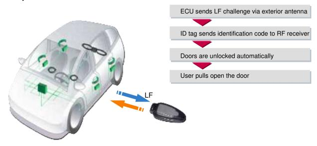
Figure 1: Principle of Communication
