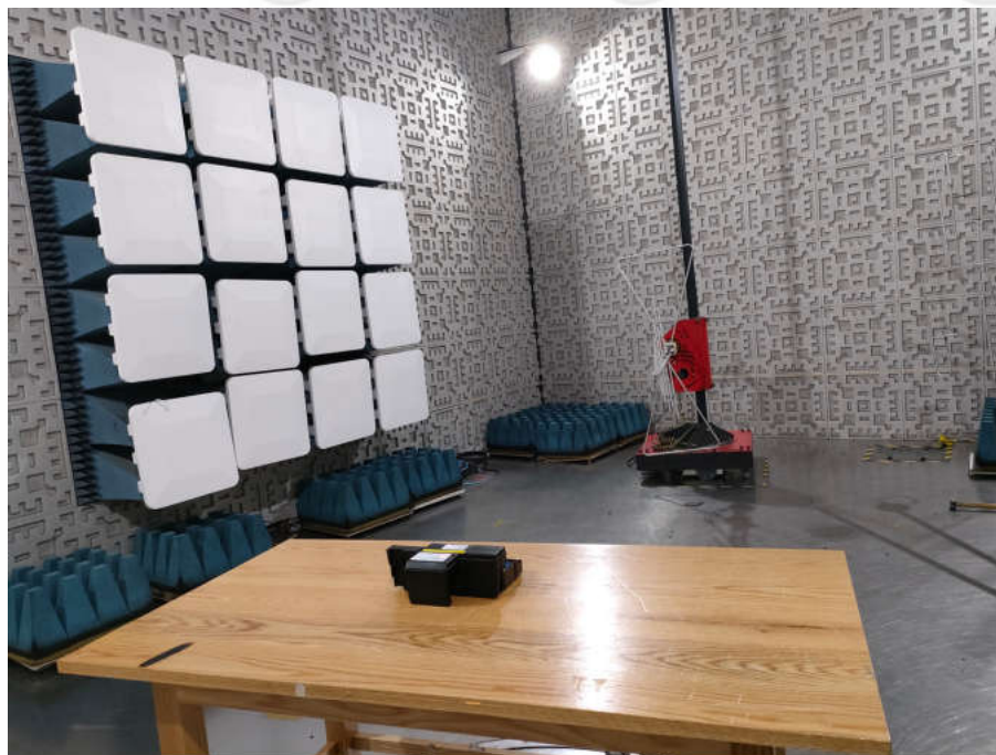
Radiated spurious emission Test Setup-1(Below 1GHz)
