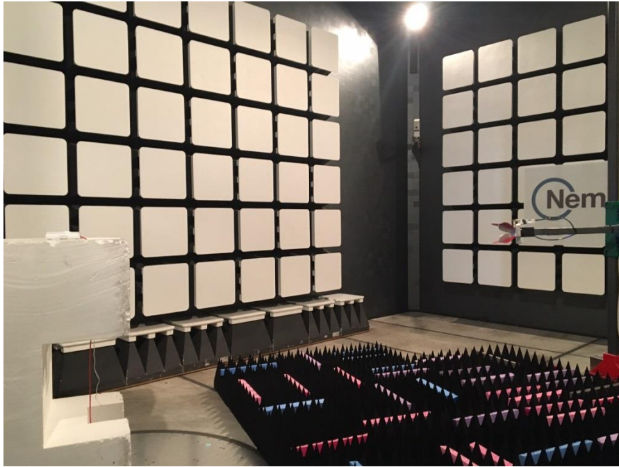
Figure 8.1-17: Radiated – Undesirable (unwanted) emissions setup photo – above 1 GHz
